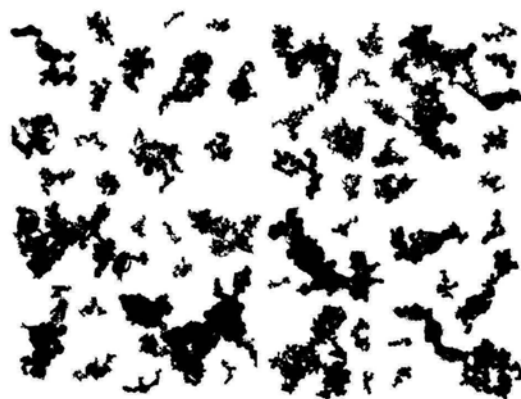
Figure 5 Reference particles for soot modeling selected from microscopic images. The largest particle has D \sim 3 \mu\text{m} .
