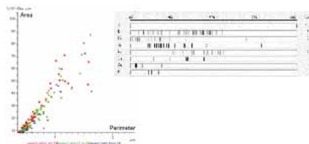
Figure 4 Example of particle data. Scatter plot of area vs perimeter (left), and a quant bar summarizing all of the elements and their concentrations (right)
