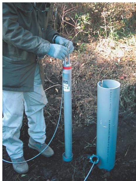
Photo 2.1.3.1 Pinnacle tiltmeter model 5000 and observation well of Araso station.
