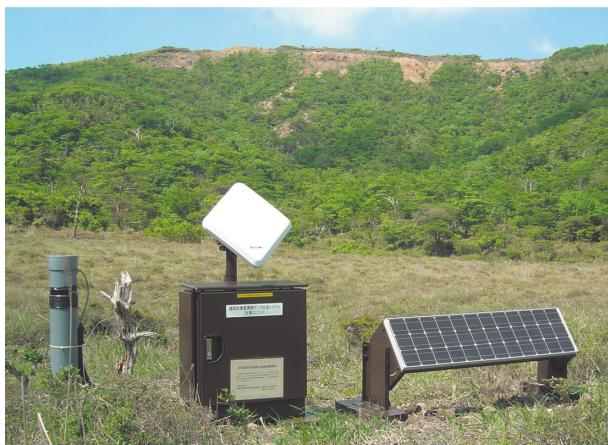
Photo 2.1.3.2 Tilt observation system at Shinmoe station.
