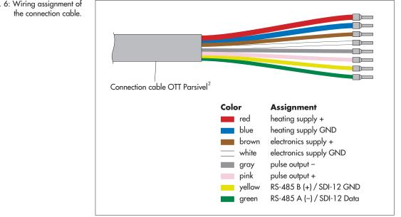
The green and yellow cable is assigned either to the RS-485 or SDI-12 interface. The selection is carried out during setup via the OTT Parsivel user software ASDO or a terminal program. Both of these wires are assigned to the RS-485 interface at the factory.
