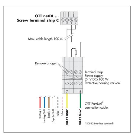
Fig. 10: Connecting the OTT Parsivel<sup>2</sup> to an OTT netDL via the SDI-12 interface.
