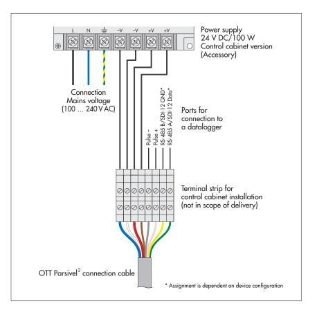
Fig. 17: Connecting power supply control cabinet version to the OTT Parsivel<sup>2</sup>.
