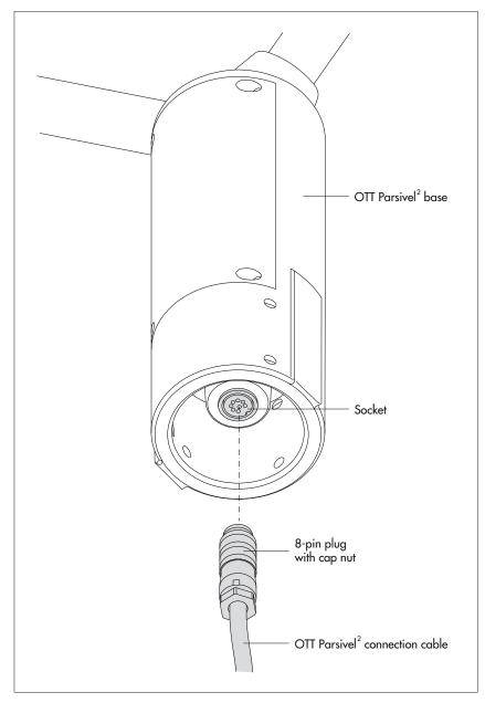
Fig. 4: Connecting the connection cable to the OTT Parsivel<sup>2</sup> base.
