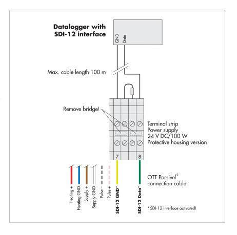
Fig. 9: Connecting the OTT Parsivel<sup>2</sup> to a datalogger via the SDI-12 interface.
