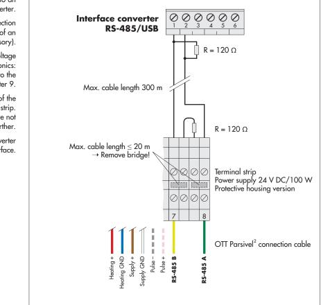
Fig. 15: Connecting the OTT Parsivel<sup>2</sup> to an RS-485/USB interface converter.
