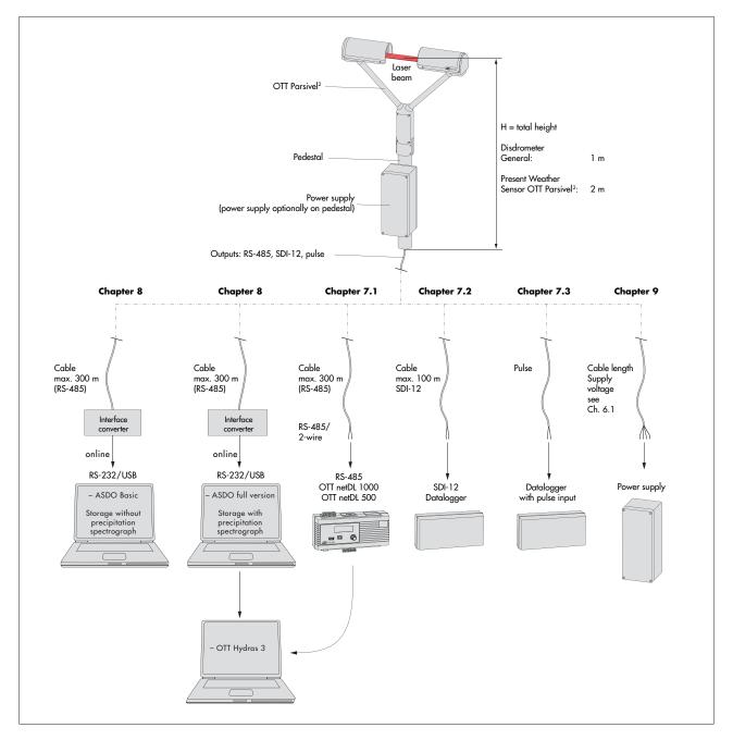
Fig. 2: Connection options for the OTT Parsivel<sup>2</sup>.
