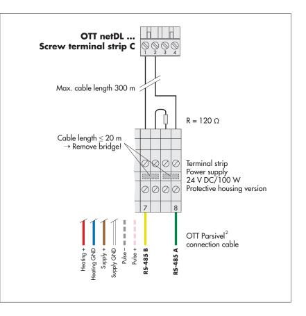
Fig. 7: Connecting the OTT Parsivel<sup>2</sup> to the OTT netDL via the RS-485 interface.
