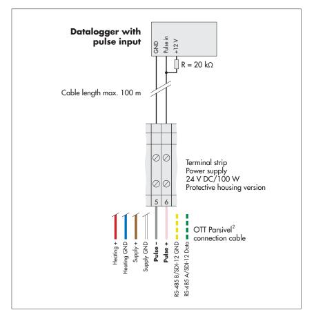
Fig. 12: Connecting the OTT Parsivel<sup>2</sup> to the datalogger with pulse input.
