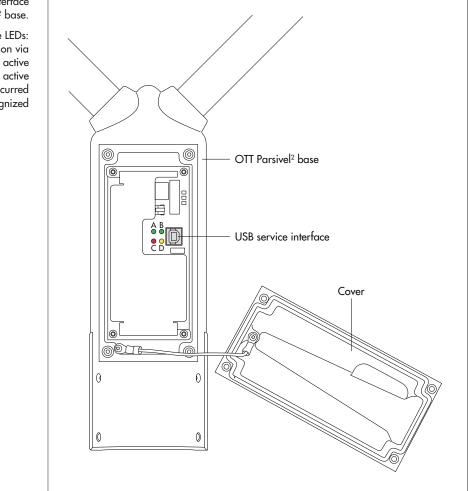
Fig. 16: Position of the USB service interface in the OTT Parsivel<sup>2</sup> base.
