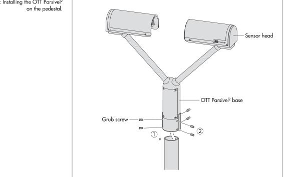
Fig. 5: Installing the OTT Parsivel<sup>2</sup> on the pedestal.
