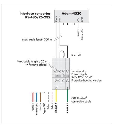
Fig. 14: Connecting the OTT Parsivel<sup>2</sup> to an ADAM-4520 RS-485/RS-232 interface converter.
