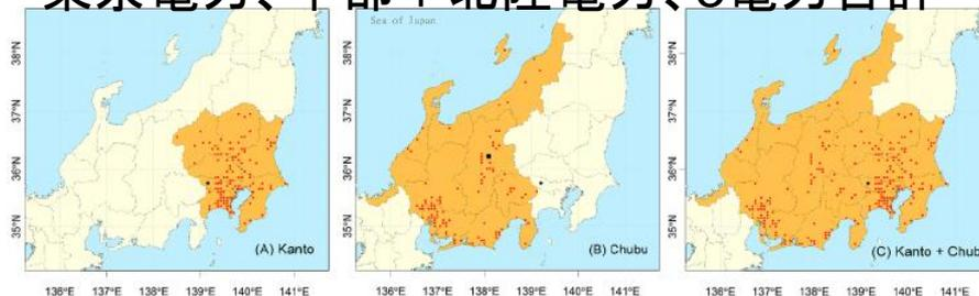
Figure 2. Target areas (in orange) with their respective PV systems' locations (in red) regarded in the regional forecasts of PV power. Asterisks (\*) indicate the Tokyo administrative area. Filled squares (■) indicate the Nagano Prefecture.
