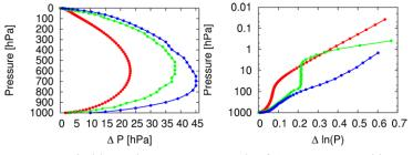
**Fig. 1:** Vertical layer placement. An example of GSM L100 created by the procedure described in the text (red), GSM L60 in operation (green), and GSM L40 which was in operation until 2007. Profiles of  $\Delta p_{k\,n-l/2}$  (left) and  $\Delta \log(p_{k-l/2})$  (right). Note that  $\Delta \log(p_{k\,-l/2})$  at the top is infinity.
