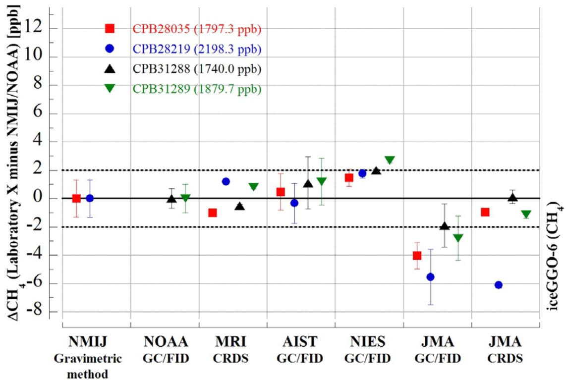
**Figure 7.** Differences (Laboratory X minus NOAA/NMIJ) of CH<sub>4</sub> concentrations for each round-robin cylinder measured during the iceGGO-6. The error bars represent the ± measurement precision reported by each laboratory, although the error bar of the NMIJ indicates the ± expanded uncertainty of the gravimetric method ( $k = 2$ ). The dashed lines around the zero line identify the WMO recommended criterion (±2 ppb) for CH<sub>4</sub> measurement compatibility.
