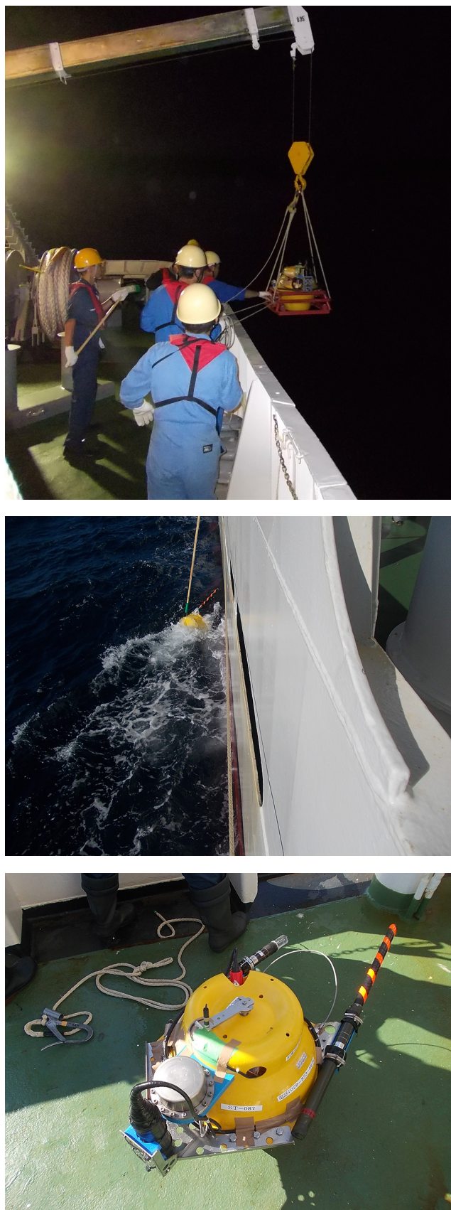
Photo 4 Deployment and recovery operations for pop-up OBPG. Pressure gauge being deployed (top), popped-up (middle), and recovered (bottom).
