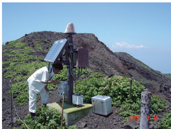
Fig. 2 Measuring microgravity with gravity meters at G22 on Mt. Miharayama, on January 14, 2006.
