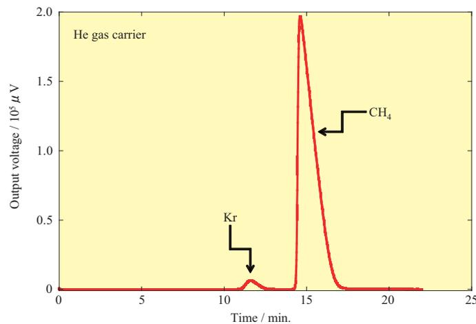
Figure 2.13 Chromatogram of stable Kr determination
