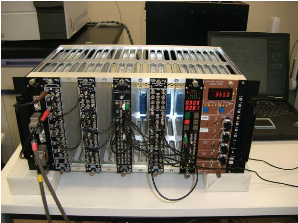
Figure 2.11 Activity counting unit (Electronics of the counting system)
