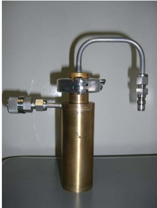
Figure 2.5 Water adsorbent tube
