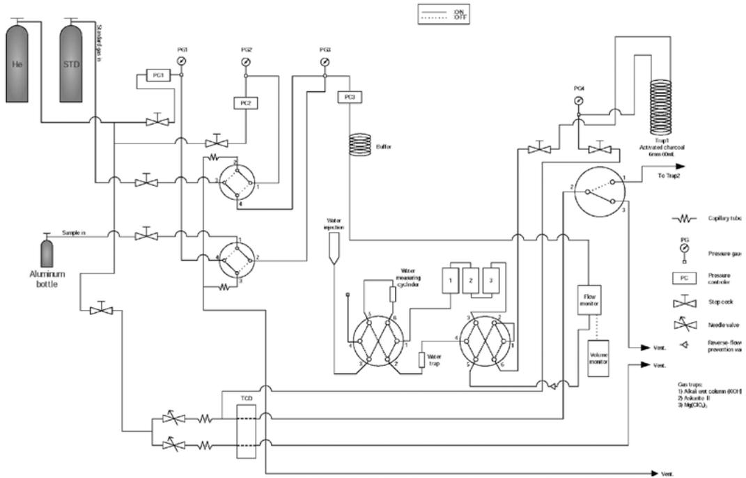
Figure 2.7 Schematic flow chart of pre-treatment unit
