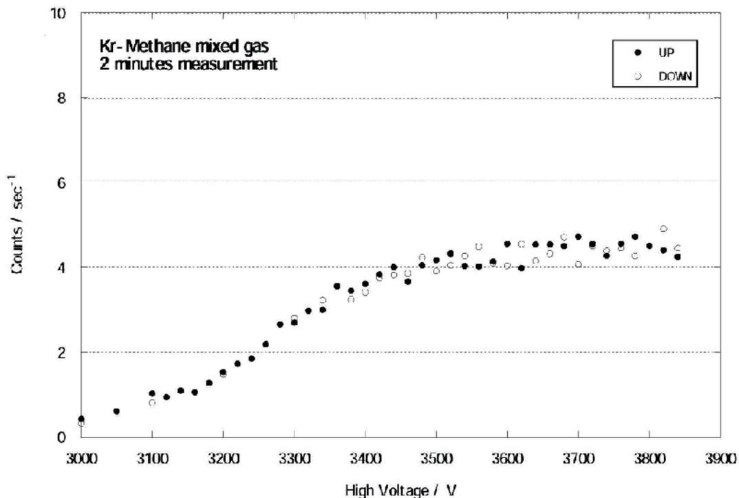
Figure 2.10 Plateau curve of the center proportional counter
