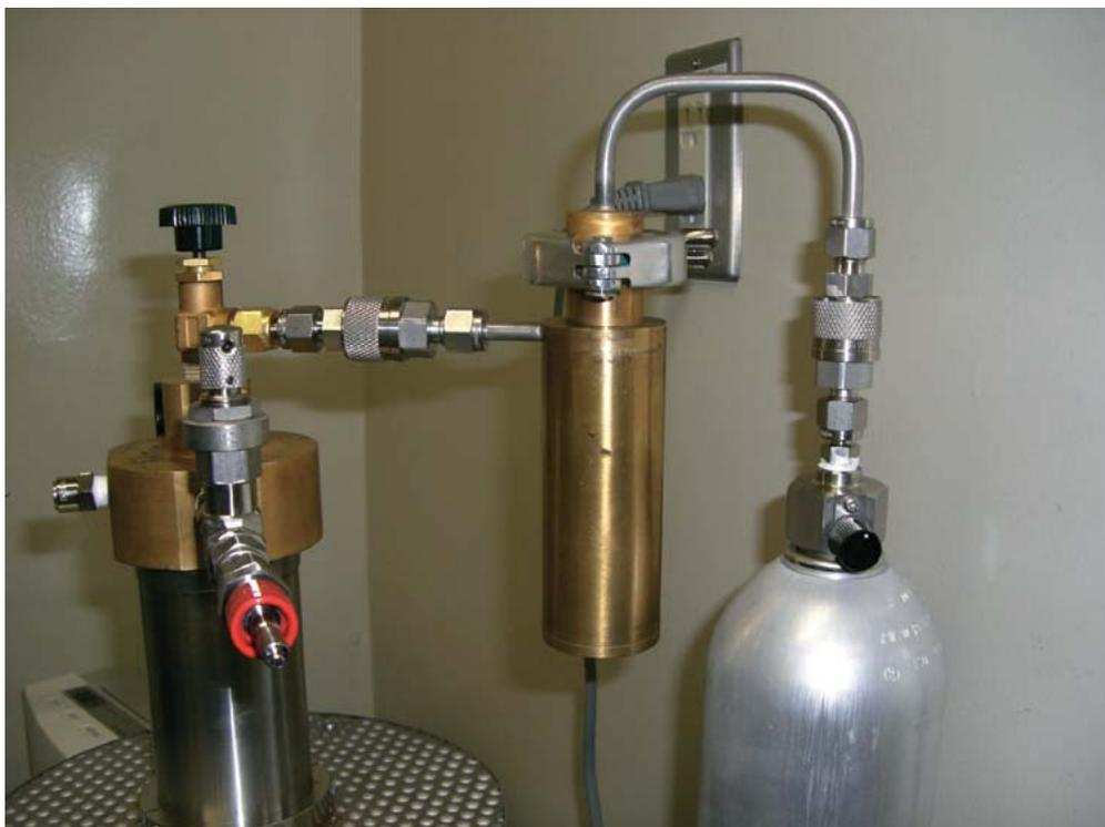
Figure 2.6 Transfer of sample gas
