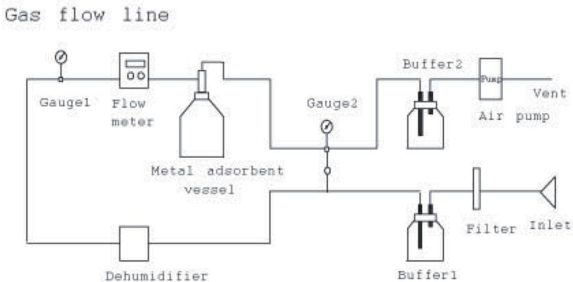
Figure 2.2 Diagram of sampling apparatus
