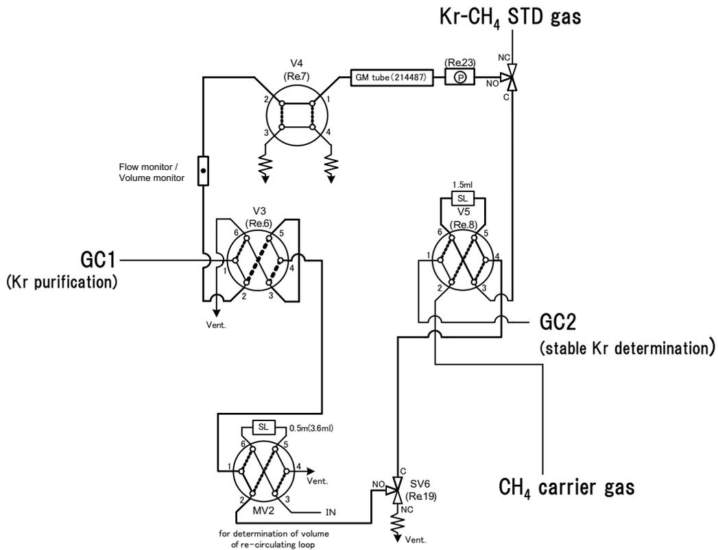
Figure 2.9 Schematic flow chart of recirculating loop
