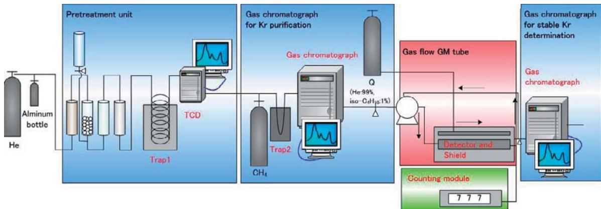
Figure 2.1 Schematic diagram of the  $^{85}\text{Kr}$  measurement system
