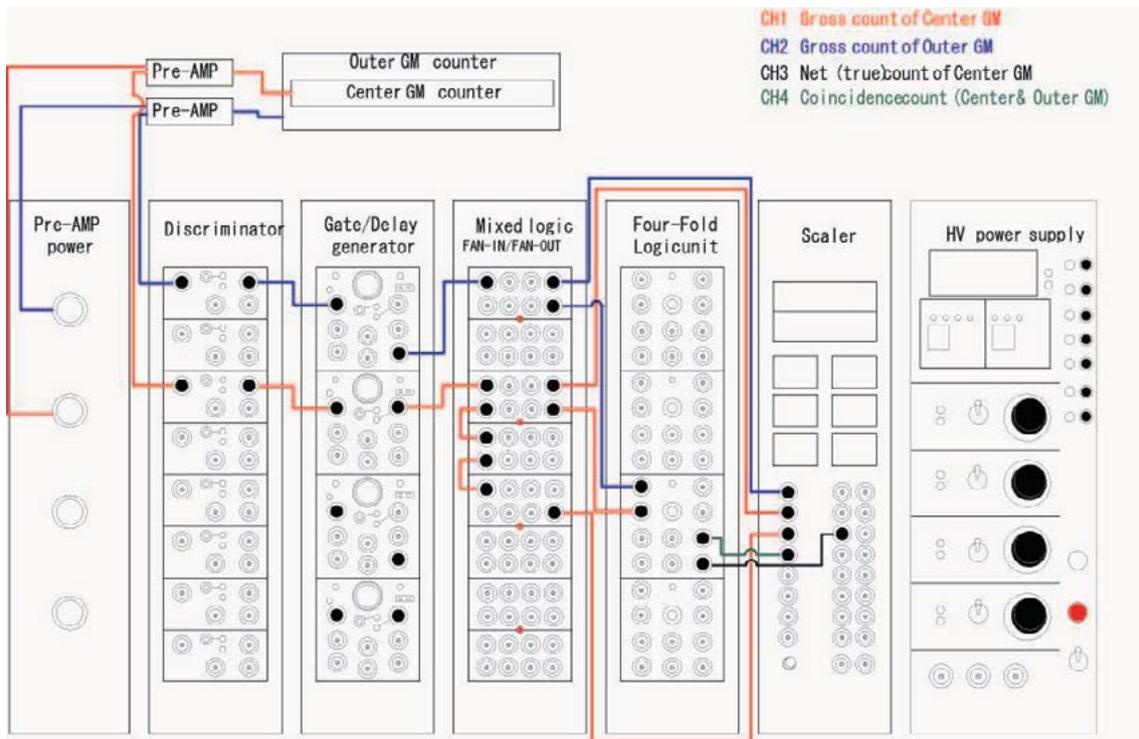
Figure 2.12 Diagram of signal cable connection
