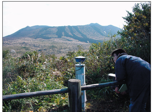
Photo 2.3.2.2.1 Scenery of repeated GPS observations at G25. The disk-shaped object on the pillar is the GPS receiver. The volcano in the background is Mt. Mihara.
