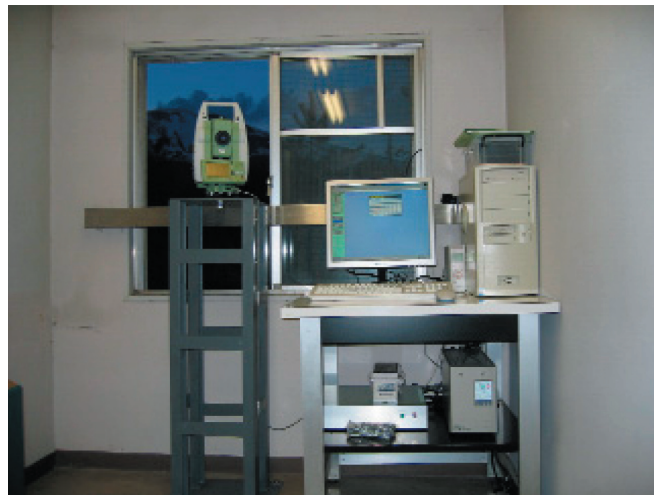
Photo 2.2.1.3 Automatic EDM system installed at KWS for measurement of ground deformation at Asama volcano.
