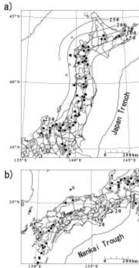
Fig. 1.5.1 Distribution of epicenters of low-frequency events in the Japan Islands around the Moho discontinuity determined by JMA (Japan Meteorological Agency) from September 1999 to February 20, 2003, in a) Eastern and b) Western Japan. Open circles designate events away from active volcanoes, and closed circles designate events within 10km of active volcanoes. Active volcanoes are depicted by gray triangles. Top depth contours of a) the Pacific Plate and b) the Philippine Sea Plate are also represented with depth by km.
