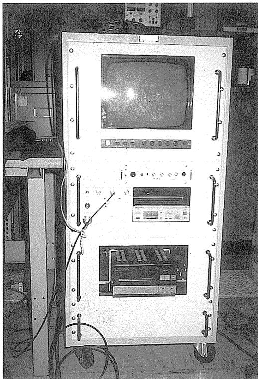
Photo 1.1.2 Photograph of data acquisition system of the CPVS ; TV monitor, time code generator, VTR and hard copy processor.
