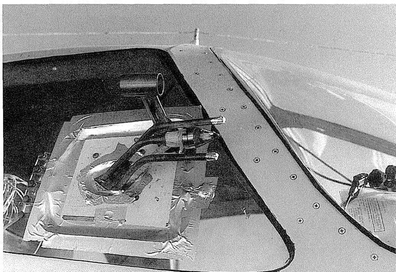
Photo 1.3.2 Inlet installed in an aircraft.
