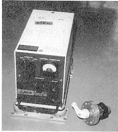
Fig. 4.8 EG & G Hygrometer Model 137 aircraft sensor assembly.
