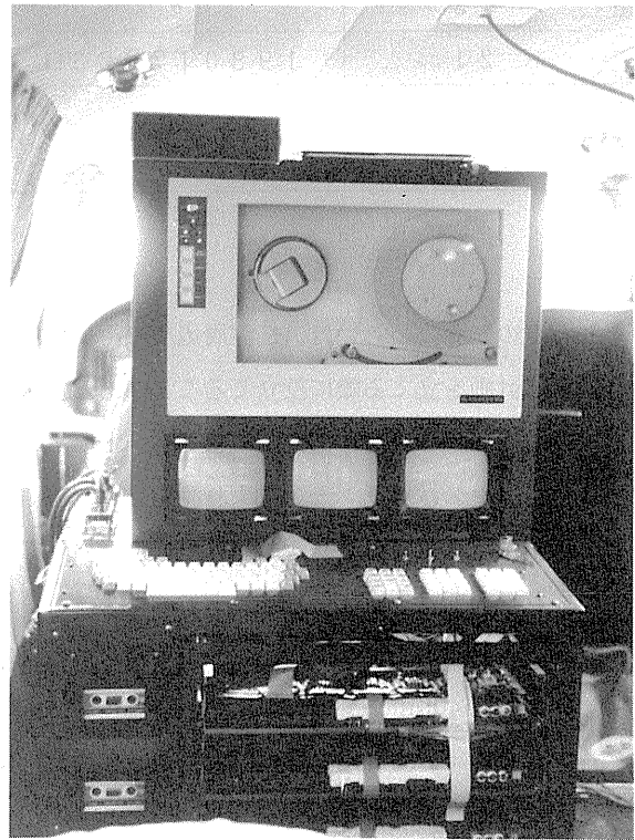
Fig. 4.20 Data acquisition system in 1981. Data and tracks are displayed on the CRT displays.
