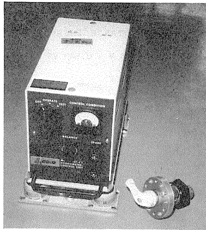
Fig. 4.8 EG & G Hygrometer Model 137 aircraft sensor assembly.
