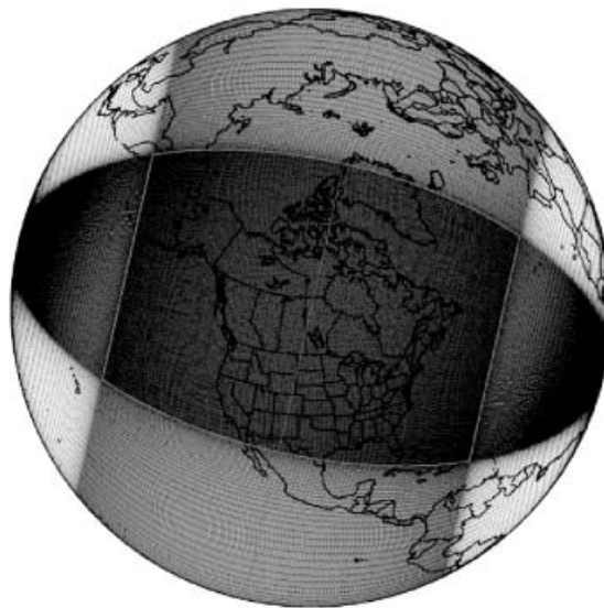
Fig. 5. Domain of variable grid GEM at MSC. By courtesy of Jean Cote of RPN.
